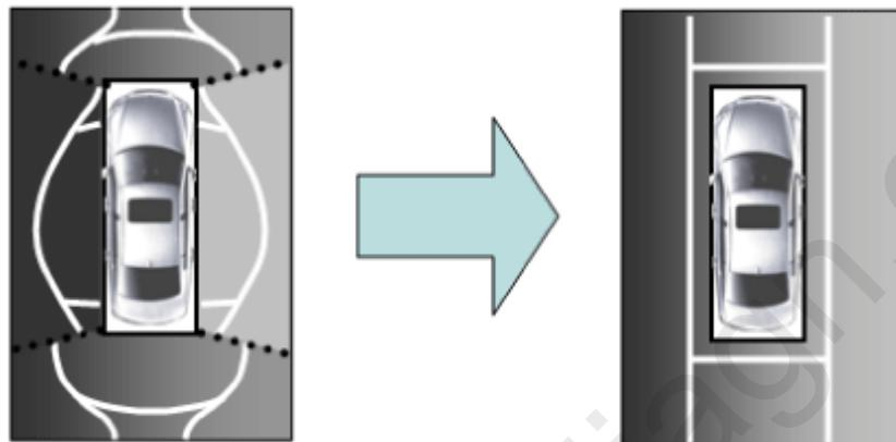
This system displays the video images from ultra optical cameras mounted on 4 sides of the vehicle, on the Head Unit Screen. It shows 360 degrees sky-view image of the vehicle's surrounding area, as well as various other view modes.
